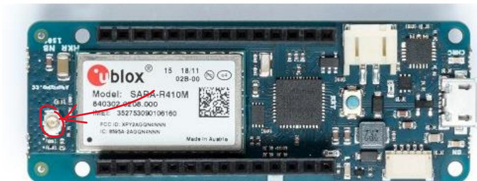
Gently put the connector at the end of antenna's wire on top of the board's antenna port and press down. Once done, it should look like below:
