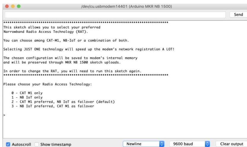
Enter 2 in the test box at the top and press send. This will activate option 2, CAT M1 preferred, and narrow band IoT as failover. Once you see the done message, you're ready to test your connectivity.
