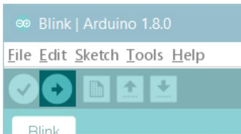
The sketch will be compiled and then uploaded. After a few seconds the bottom bar should show *Done Uploading*. You have successfully set up your MKR NB 1500 board and uploaded your first sketch.
