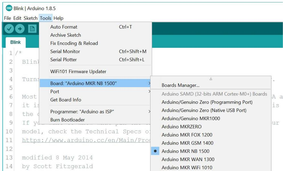
Once selected open the port menu just below that and select the serial port which is occupied by the board.
