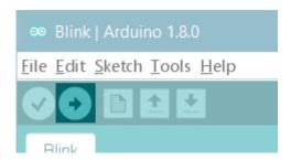
The sketch will be compiled and then uploaded. After a few seconds the bottom bar should show Done Uploading.
